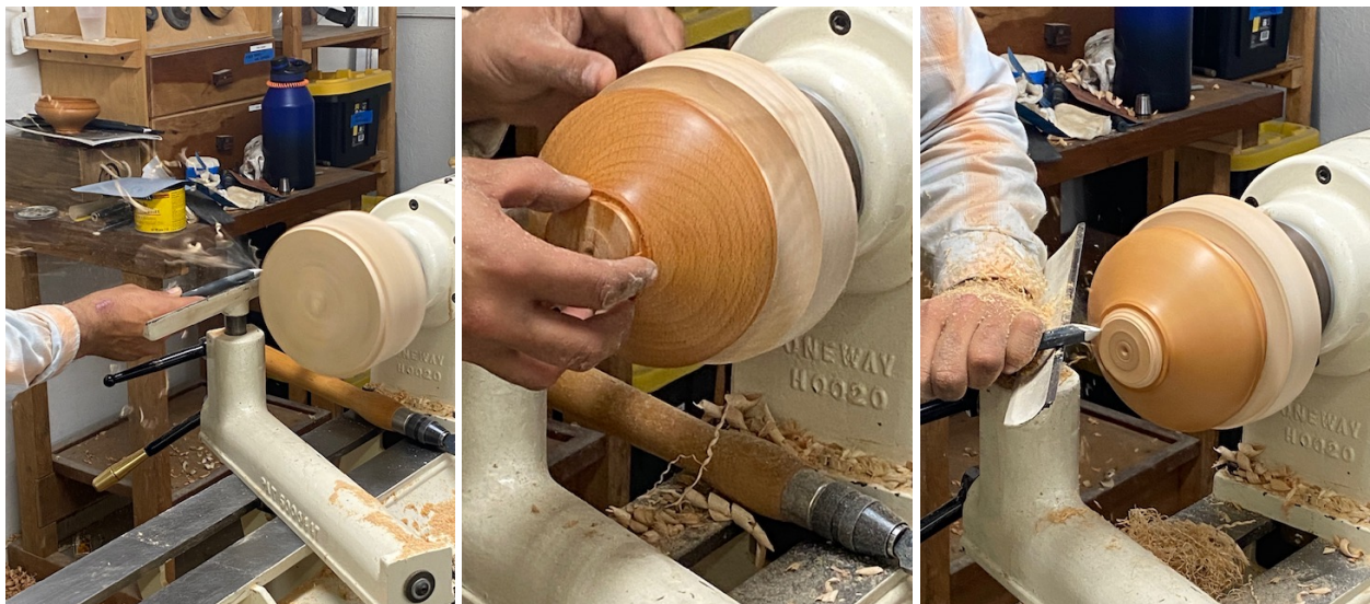
REMOVING THE TENON – JAM CHUCK, CHECKING THE FIT
