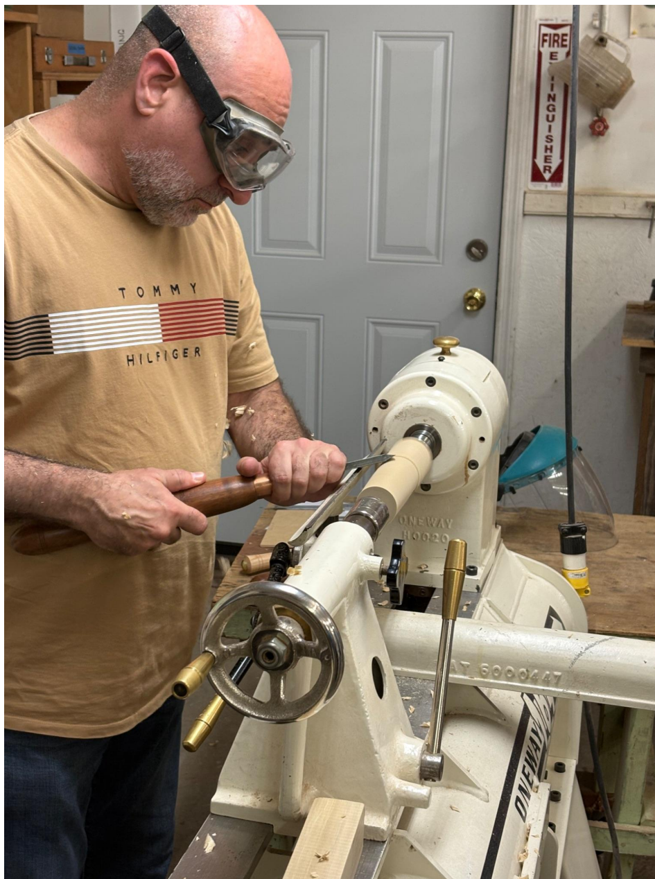
Rounding poplar block with Skew chisel
